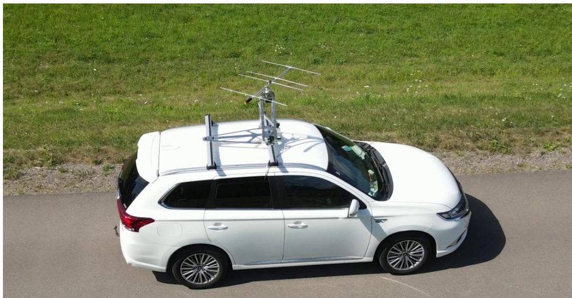
CAR with our 4-element Yagi antenna in action.
