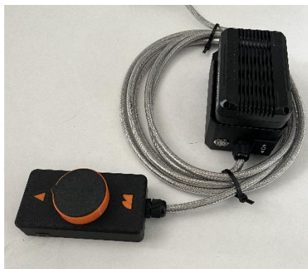
Control unit with rotary dial and battery unit with power button and (un-) fold button.
