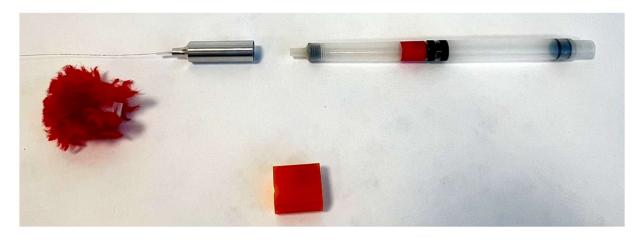
Insert the Transmitter into the aluminum tube (SG-k) like shown on the image above. Make sure that the aerial of the transmitter is not jammed.
