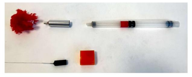
The Transmitter is activated by removing the red rubber box. Now it is time check the transmitters frequency using all receivers which will track it. Each receiver might have an offset. Tune to the best signal and note it for all receivers.
