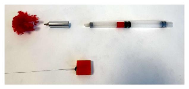
Our transmitter is shipped in a little red box, within a plastic package – written on the package is the frequency of the transmitter. Tune your receiver to that frequency. If you use a receiver in USB mode, remember that you must stay below that stated frequency.
