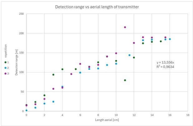
The pattern is clear – the longer the aerial, the higher the detection range. Keep in mind, that the transmitter was covered by 0.5m of soil. Assuming a linear pattern (simple linear regression model), we lose 13,6 m detection range per cm cut ( $R^2 = 0.96$ ) in this setup with the transmitter 0.5m underneath the ground.
