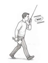
First, we walked in a straight line until we lost the signal. Then, we retraced our steps along that line for a few metres until we could hear faint but clear beeps constantly. This was the most difficult part of the experiment and, again, this is just an estimate. This position was marked with a sign indicating the length of the transmitter aerial. We used a tape measure to record the distance from the transmitter's hole to the marked point.
